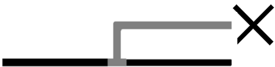
Rubber conductor not removed
