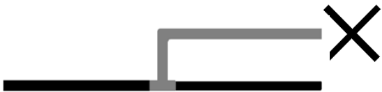
Rubber conductor not removed
